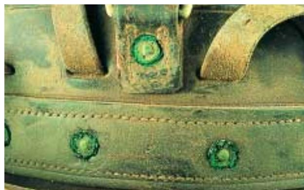
Copper corrosion products on studs of a straitjacket.
