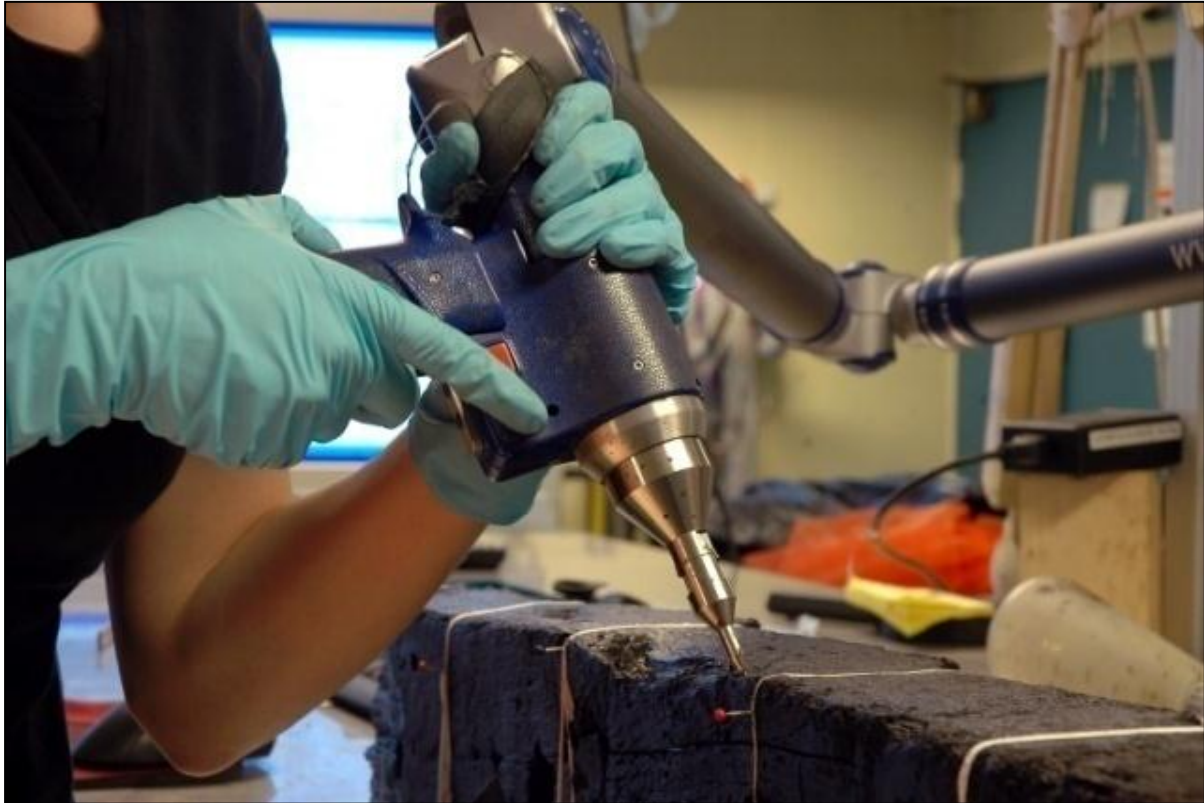
Figure 4. FaroArm probe with a pistol grip in use. By pressing the red or green button while holding the tip firmly against the object, the operator chooses where the point should be set. Photo: T. Falck/NMM.
