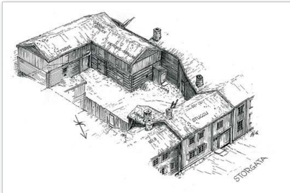
36: Rasmusgården with outbuildings: cowsbed, owner's stable and stable for travellers. Hayloft on the first floor. Drawing by Sverre Ødegaard.
